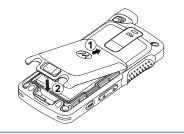
3 Slide battery latch into lock position.
